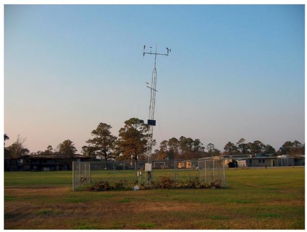
**Temperature** (soil - 5 depths and above the surface at 1.5, 2, 9.5, and 10 m).
